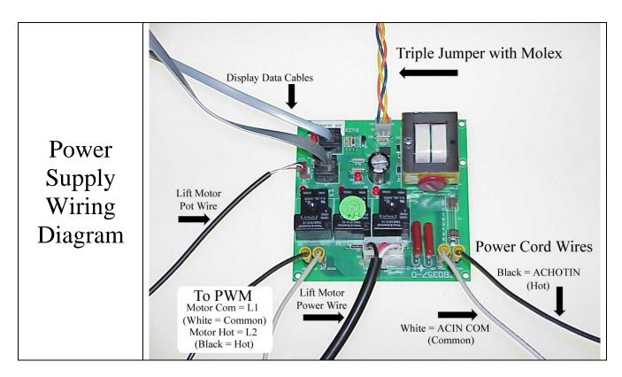
Pay close attention to the Power Cord wires that run from the end of the AC Power Cord to the Power Supply board. The black wire (hot) must be connected to the spade marked "ACHOTIN" (AC Hot In). The white wire (common) must be connected to the spade marked "ACIN COM." If the Power Cord is not connected properly to the Power Supply, the board will be permanently damaged.
